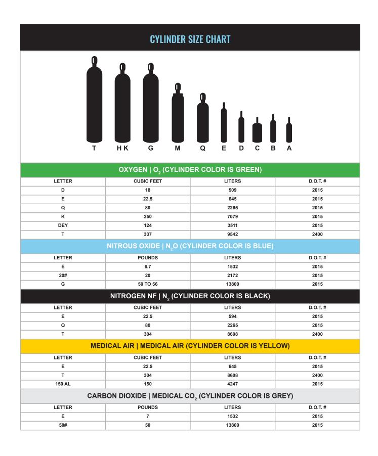
Pressure & cubic feet varies with gas type & molecule compound
